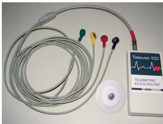
Figure 2. Recording device (Televet 100<sup>®</sup>) with 4 electrode cables (green, yellow, red and black) and a self-adhesive electrode.
